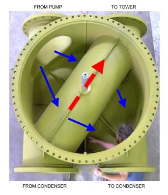
PLUG TURNS TO REVERSE HEAT EXCHANGER FLOW
